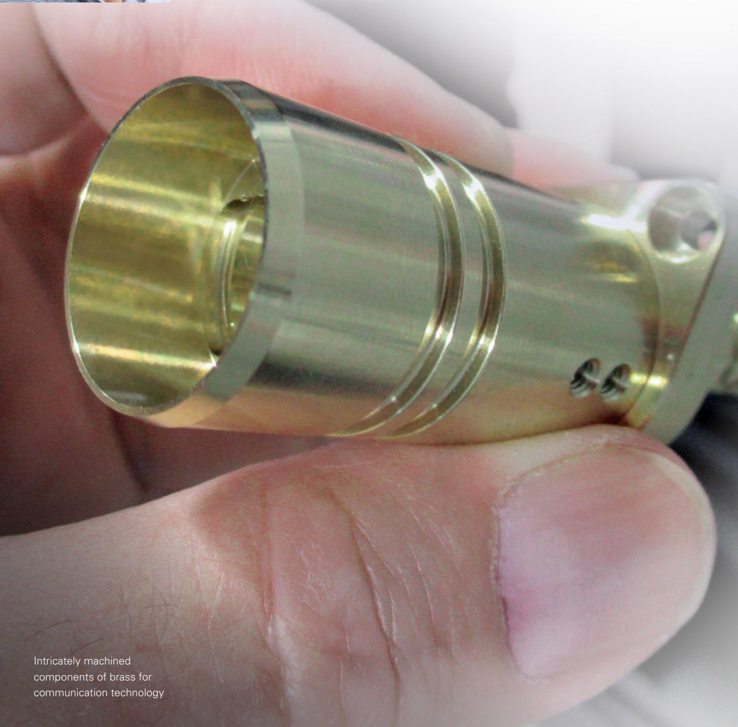
Intricately machined components of brass for communication technology
