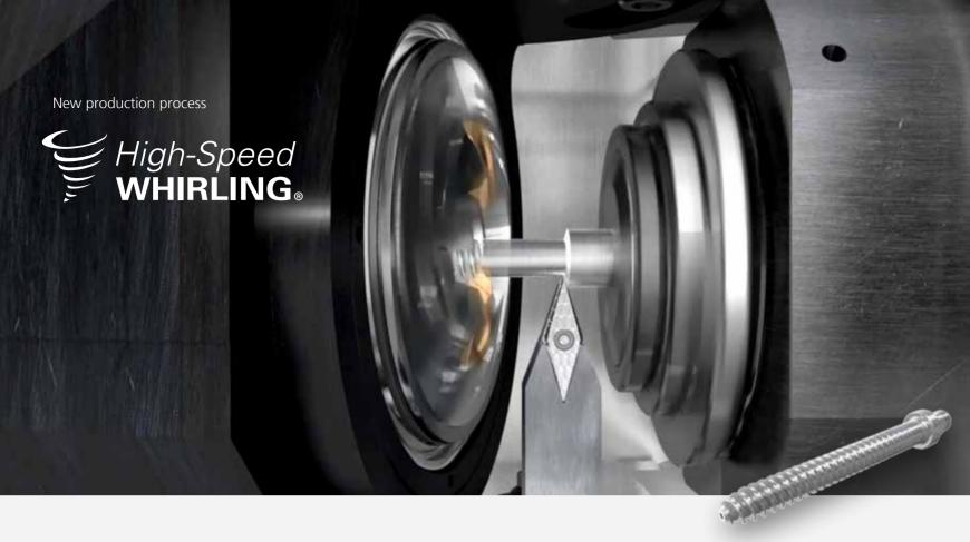
The high-speed whirling technique was developed for the production of bone screws with simultaneous turning and whirling operations. It offers considerable advantages for the manufacture of thread-type components, which are reflected in a reduction of production times, costs and an increased tool life.
