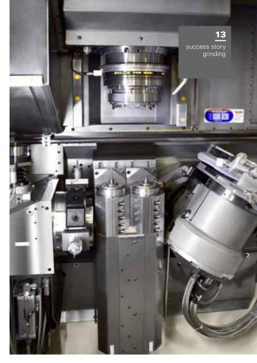
The operator can always use the particular cheaper technology due to the process combination turning/grinding.
