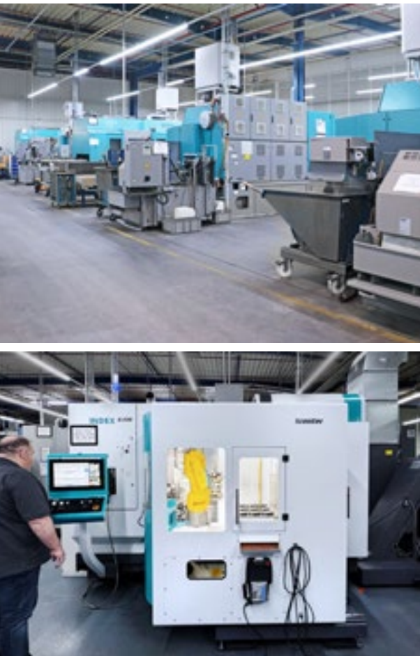
Left: A look down the INDEX aisle at KEB in Barntrup, where 14 INDEX turn-mill centers and vertical turning machines operate nearly around the clock. In continuous use since 2022: the INDEX G220 turn-mill center with iXcenter automation (photo below).
