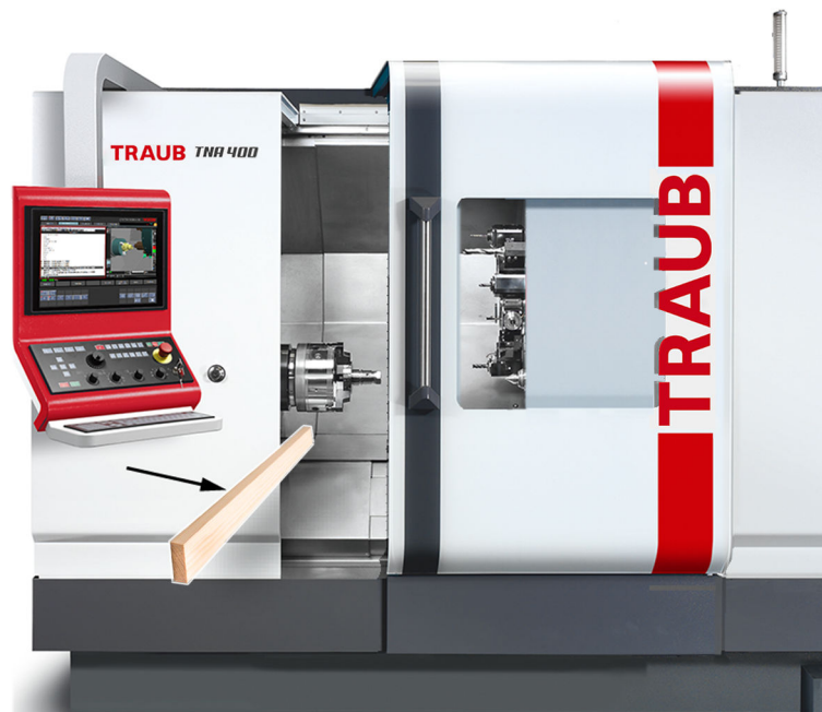
Example: Checking the obstacle detection
