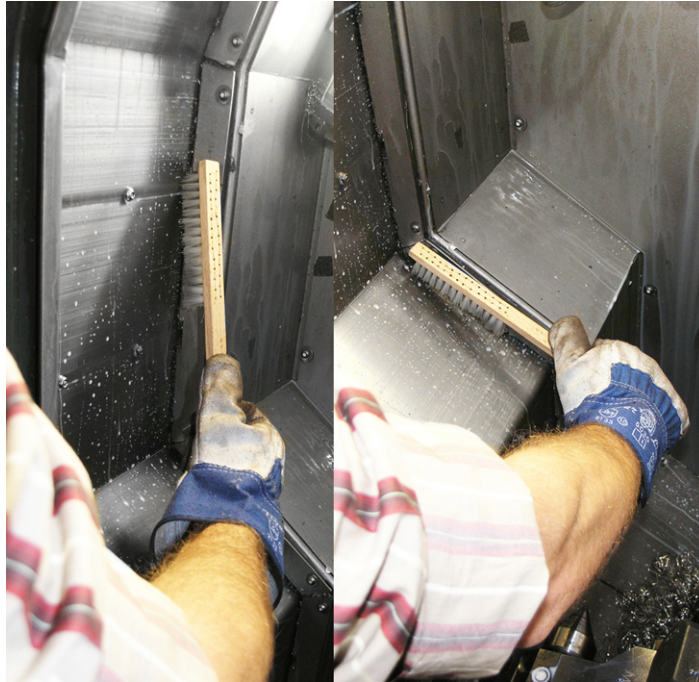
Example: 2 Sweep small chips and other debris from top to bottom using chip brooms or brushes.
